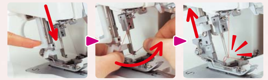
Step.1 Lower the threading lever. Step.2 Hook the thread. Step.3 Return the lever to finish threading.
