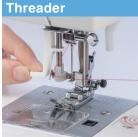
The needle threader easily threads the needle and allows you to start sewing quickly.
